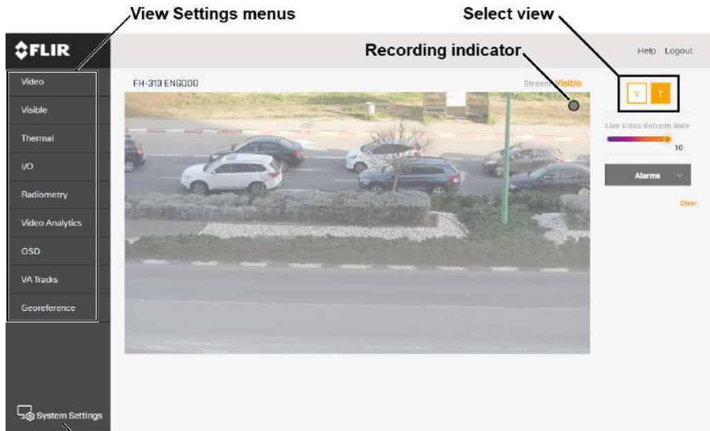
System Settings View Settings Home Page - FH-xxx R models - Users Assigned the Admin or Expert Role Visible Video Images Selected - Default Settings
