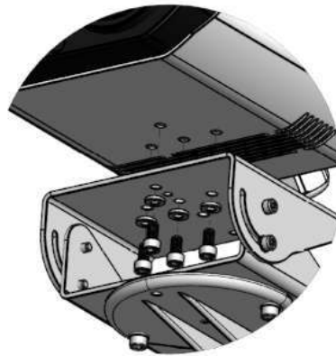
Attaching the Camera to the 421-0087-00 Wall Mount Kit
