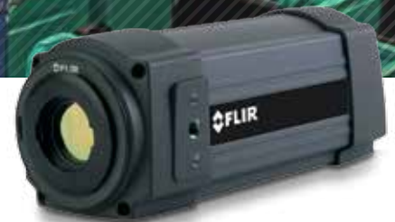
The FLIR A310 produces crisp thermal images of 320 x 240 pixels and detects temperature differences as small as 50 mK.
