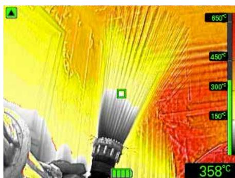
FSX ensures a clear, crisp image in every possible fire scene making the smallest of temperature differences visible. A small hot object against a cold background will have just as clear of details as the background, which is the dominating temperature range. Thanks to FSX, people can be more easily detected in hot environments like fire scenes.
