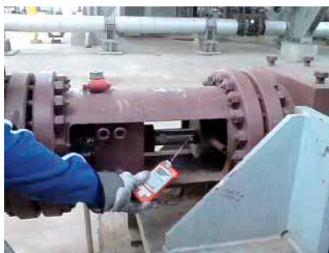
The small gas leak detected with optical gas imaging camera is quantified with a sniffer. As the concentration is below the threshold this leak does not get a high priority.
