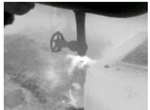
This valve is leaking ethylene, showing up as white smoke in the black hot thermal image.
