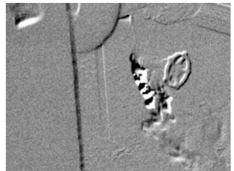
This valve is leaking ethylene, showing up as white smoke in the black hot thermal image.
