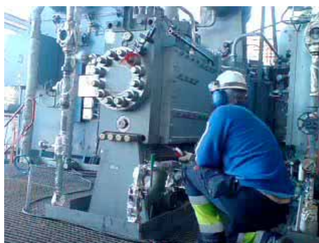
A sniffer must be held in exactly the right spot to detect a gas leak. Optical gas imaging cameras can detect gas leaks anywhere within their field of view.
