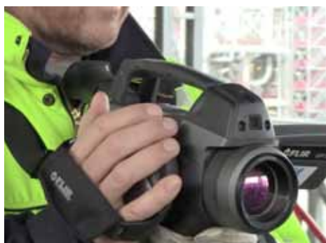
The GF306 optical gas imaging camera is compact, relatively lightweight and ergonomically designer, to prevent back and arm strain.
