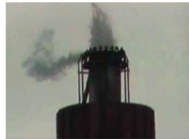
Poorly Operating / Over Steamed Flare Low Combustion Efficiency
