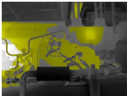
Interval alarm: Highlights all pixels with a temperature between two specified temperature levels.
