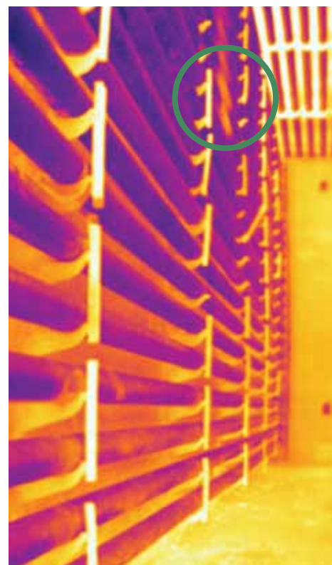
The inspection with a thermal imaging camera from FLIR revealed a hot area due to flame impingement on the tubes at start up.
