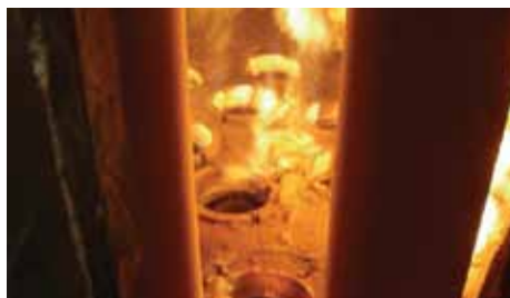
Inspection ports provide a view of internal parts, but flames, combustion gases, and ash obscure the equipment during operation. A FLIR thermal imaging cameras with a flame filter is not hindered by such obscuring.
