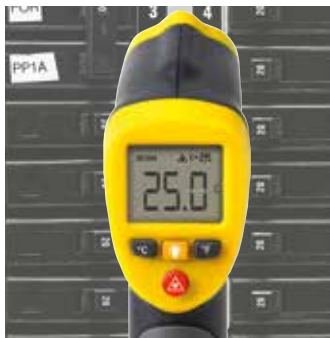
IR thermometer, temperature measurement in one spot
