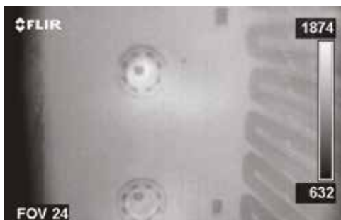
Thermal image: due to the built in flame filter the FLIR GF309 thermal imaging camera can see through flames and even measures the temperatures behind the flames.
