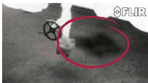
Captured gas leak from production site.
