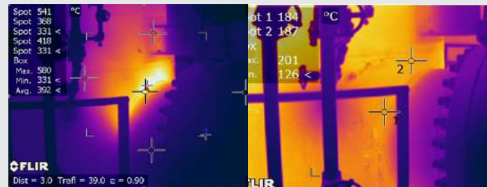
Refractory Lined Equipment Nozzle-Images before (hot spot indication) and after refractory repair (no hot spot indication)
