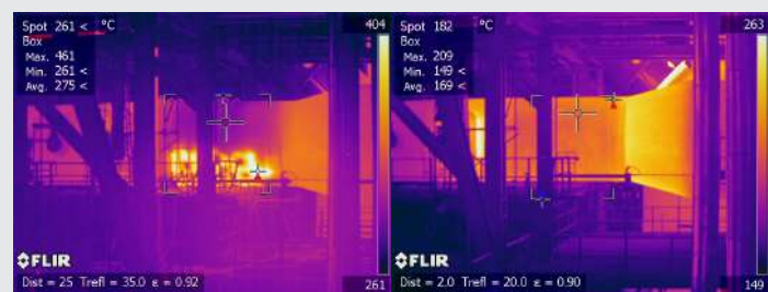
2nd Stage Regenerator Orifice Chamber-Images before (hot spot indication) and after refractory repair (no hot spot indication)
