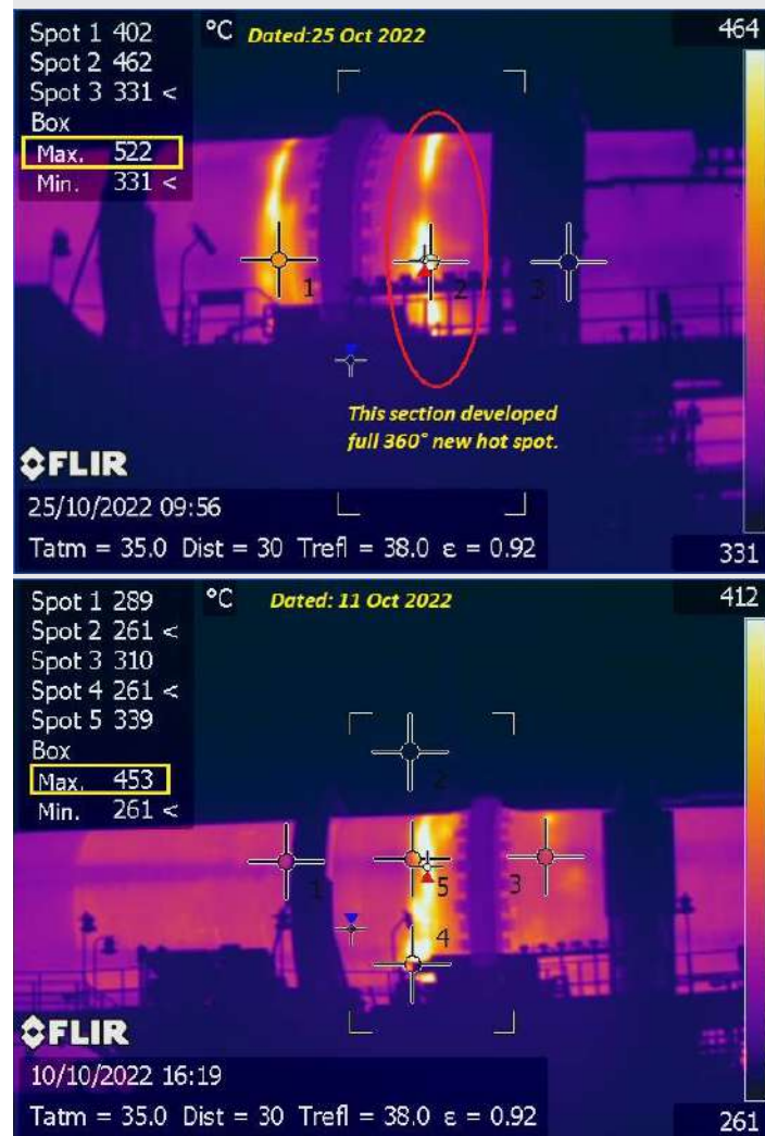
Thermography of Rotary Kiln showing hotspot caused by refractory damage.
