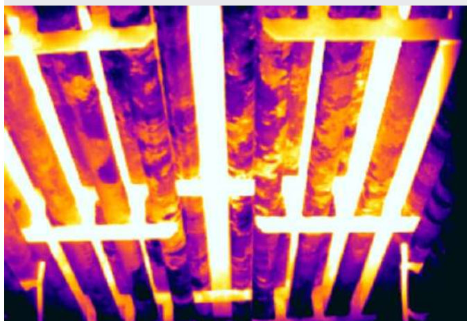
Fig. 2. External scaling on the tubes leads to a patchy appearance, both in infrared and visible light. Areas with defined edges that appear hot in the thermal image are actually not overheating..
