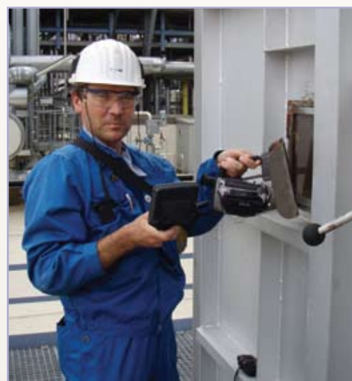
Holger Springer with his FLIR infrared camera at a furnace inspection window
