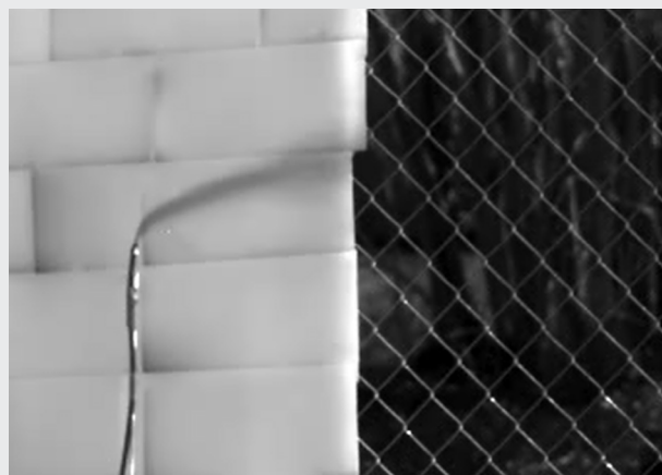
Image of a gas leak showing the effects of Delta T as the gas moves from a hot background (the wall) to a background that is ambient temperature (the fence)
