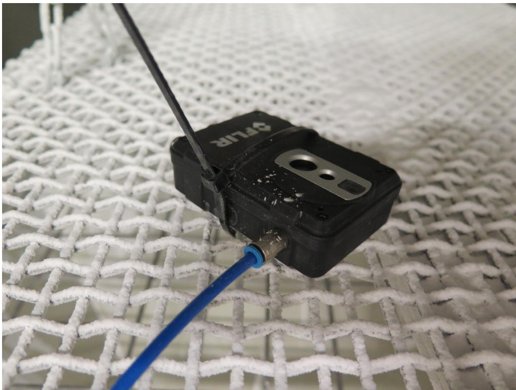
Picture 3: EUT inside the dust chamber (IP6X test)
