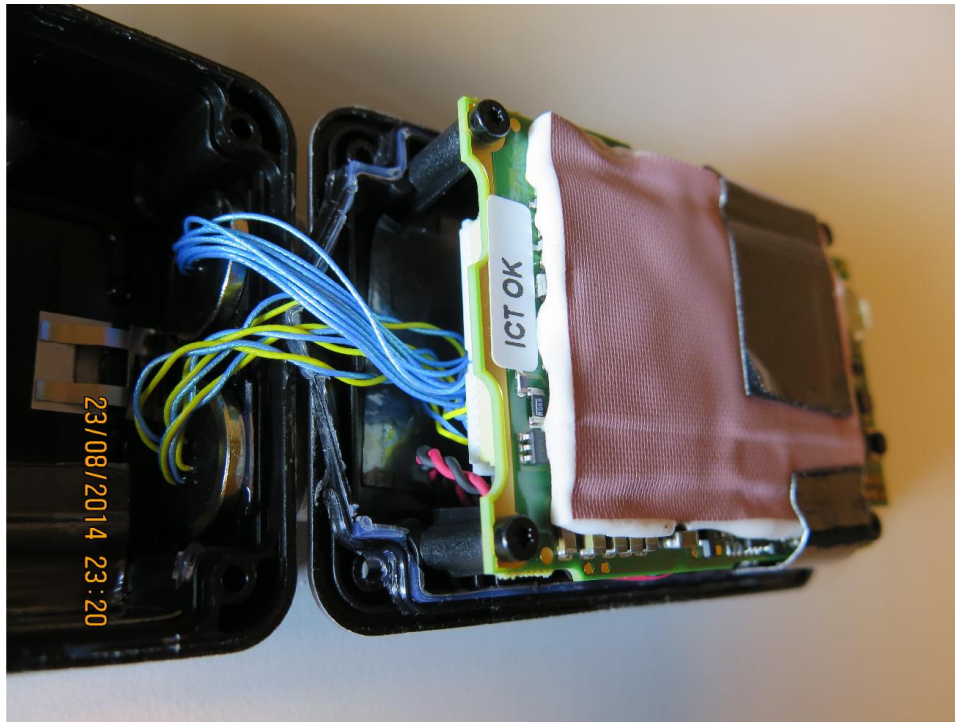
Picture 6: No dust inside EUT after IP6X test
