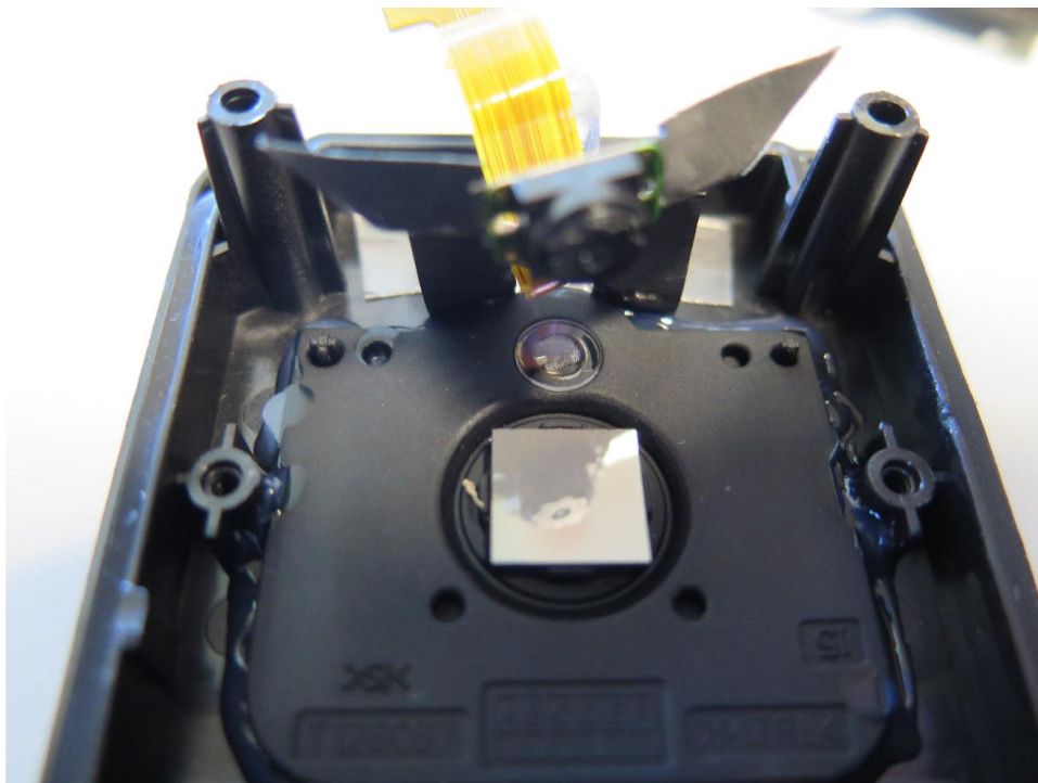
Picture 9: No ingress of water at the IR interface
