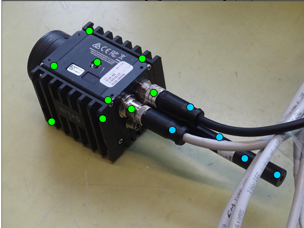
Photo 27: Contact discharge (green), air discharge (blue)
