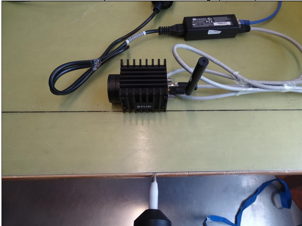
Photo 20: Example of indirect contact discharge (horizontal)
