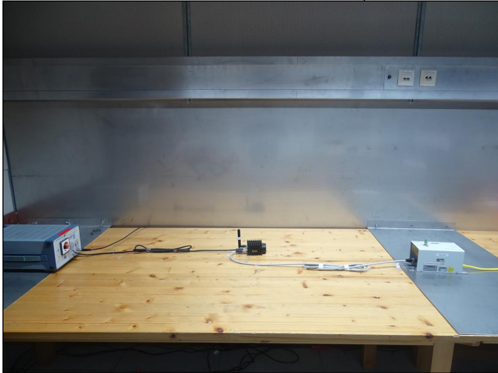
Photo 5: Conducted emissions test setup
