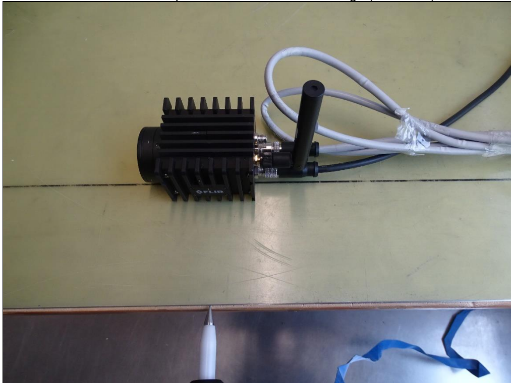
Photo 24: Example of indirect contact discharge (horizontal)
