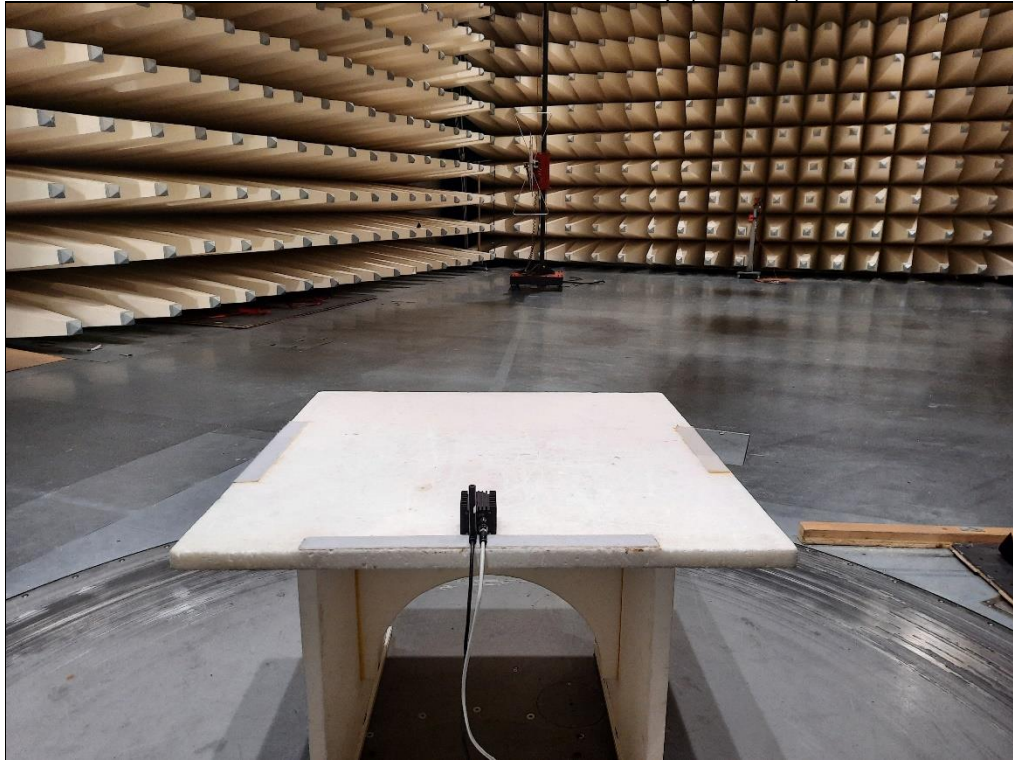
Photo 3: Radiated emissions test setup (< 1 GHz)
