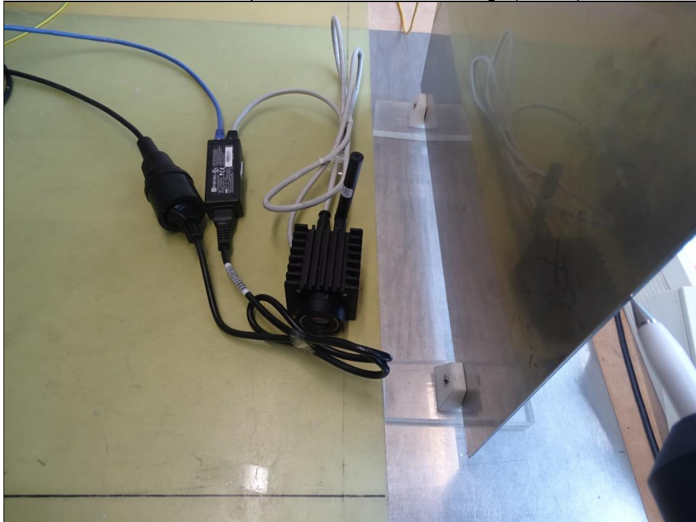
Photo 21: Example of indirect contact discharge (vertical)
