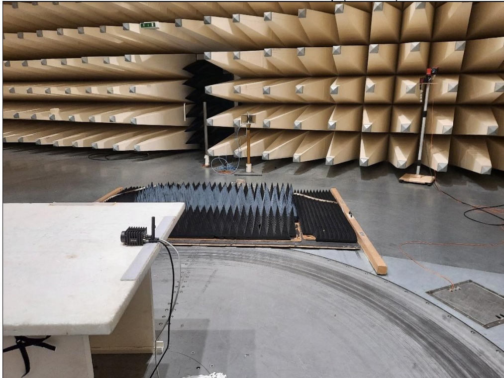
Photo 4: Radiated emissions test setup (> 1 GHz)
