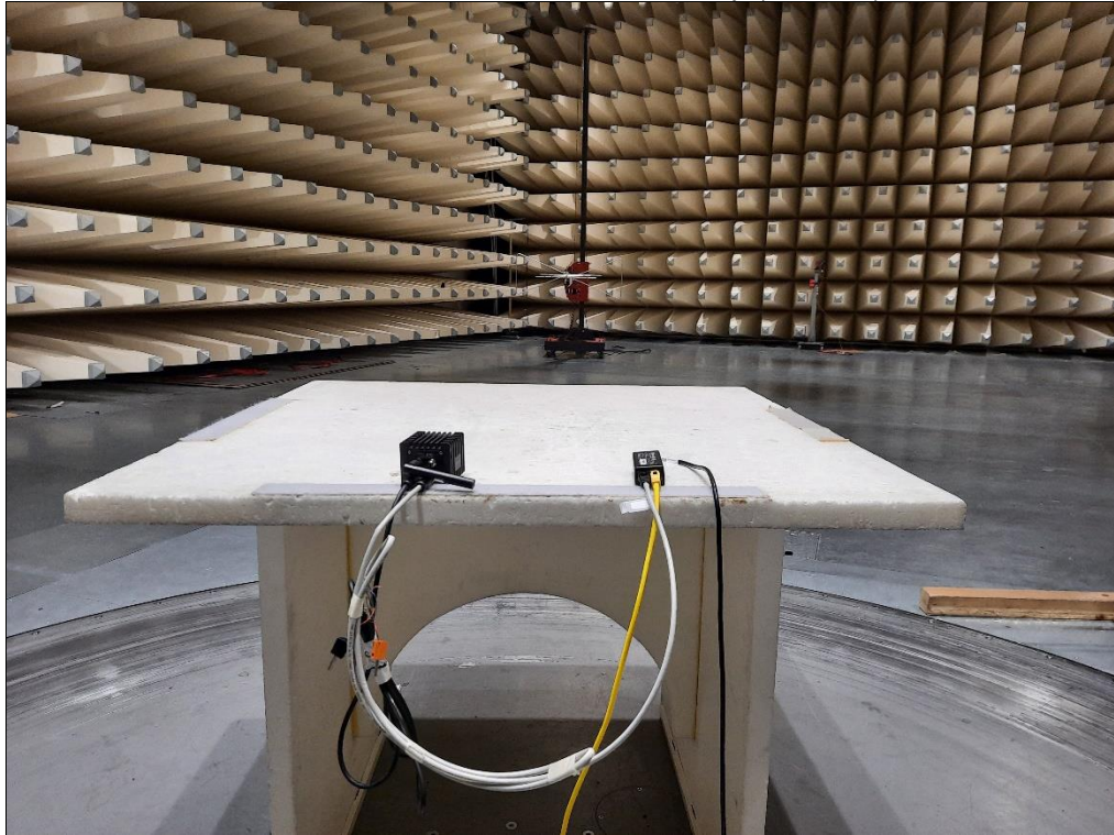
Photo 1: Radiated emissions test setup (< 1 GHz)
