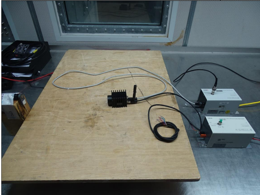
Photo 13: Example of conducted radio disturbance test setup
