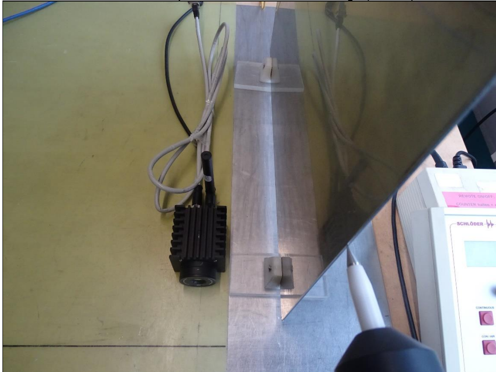
Photo 25: Example of indirect contact discharge (vertical)
