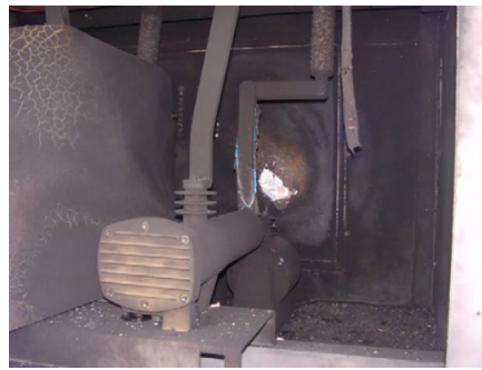
Failed Voltage Transformer Inside Circuit Breaker
